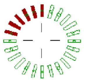
The problem with this method is that there are now six pin 1's, six pin 2's, etc. Also, there are now six components instead of just one. This is the trade off. You can inspect the device, but you have to do it as six devices. It is better than not being able to inspect it at all.
