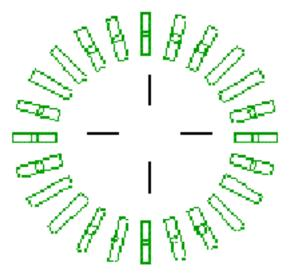
Unfortunately, the pin orientation does not survive the CAD conversion into the NDF structure. The NDF files can not handle non-orthogonal pins. The component is barely recognizable as a round component when we view it in DRAWCAD. It might look something like this real example:
